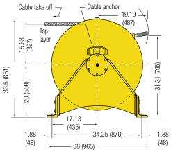
FA5T-24 with disc brake only in inches (mm)
