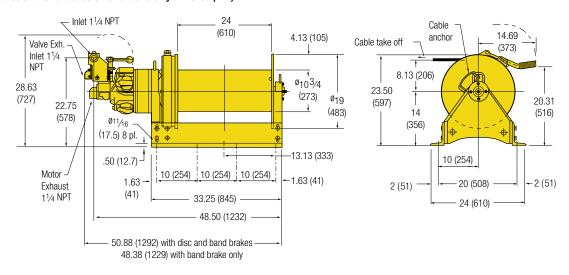
FA2-24 with disc brake only in inches (mm)
