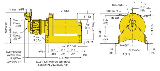
FA5-24 with disc brake only in inches (mm)
