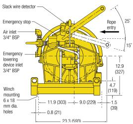
LS500RLP and LS1000RLP pneumatic winches in inches (mm)
