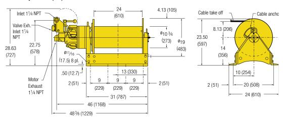
FA2.5-24 with disc and band brakes or band brake only in inches (mm)
