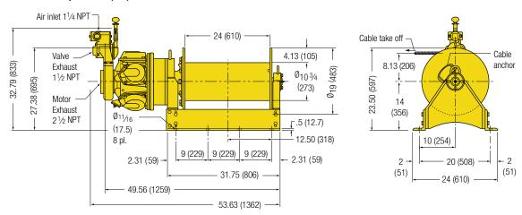
FA5-24 with disc and band brakes or band brake only in inches (mm)
